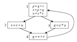
The variables which are live both at the statement in basic block 2 and at the statement in basic block 3 of the above control flow graph are
