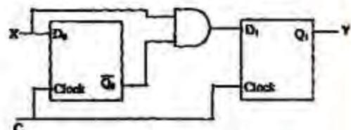
Consider the following timing diagrams of X and C; the clock period of C  $\geq 40$  nanosecond. Which one is the correct plot of Y?
