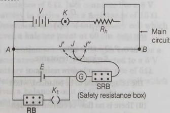
If  $l_1$ ,  $l_2$  are the balancing lengths when key  $K_1$  is opened and closed respectively and resistance R is applied in Safety Resistance Box (SRB), then internal resistance of primary cell of emfs is given
