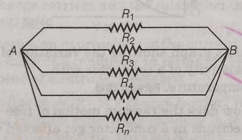
IOTE The total resistance in parallel combination is less than the least resistance of the circuit.
