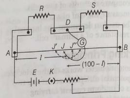
It is an electrical device used to determine the resistance and hence, specific resistance of material of given wire/conductor.
